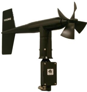
The Wind Monitor ALPINE MODEL is available with two additional output signal options. Model 05103V-45 offers calibrated 0-1 VDC outputs (0-5 VDC optional), convenient for use with many dataloggers. Model 05103L-45 provides a calibrated 4-20 mA current signal for each channel, useful in high noise areas or for long cables (up to several kilometers). Signal conditioning electronics are integrated into the sensor junction box
